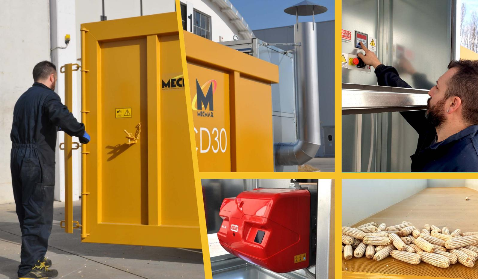
The drying process involves the channeling of hot air from the heat generator toward the shallow perforated bed. This mechanics provides the energy, heat and pressure required to extract the moisture from the cobs.
