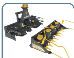
Detachable header for quicker maintenance
